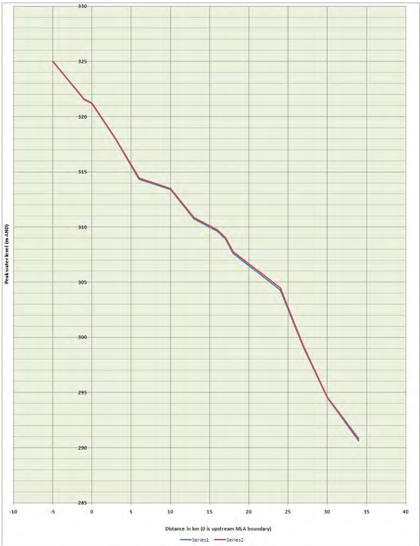
Figure B-5 Longitudinal section of the 1000 and 3000 year ARI peak flood levels for the developed case.
